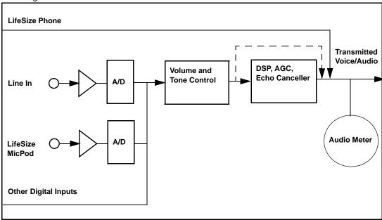
The dotted line illustrates the audio path when *Microphone In (No AEC)*, *Line In 1 (No AEC)*, or *Line In 2 (No AEC)* is selected as the active microphone. This mode is useful for setting up system gains but should never be used during calls unless the installation includes audio inputs with external AEC. Echo may occur if no AEC is employed.
